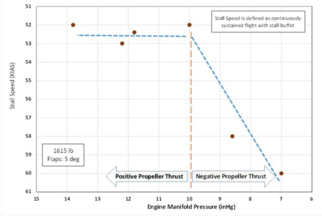
Figure 5, Effect of Propeller Thrust on Stall Speed
