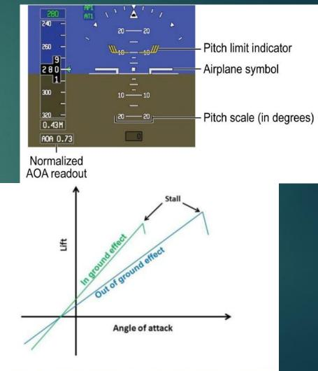
Figure 3, Critical AoA Change in Ground Effect, from NTSB report on G-650 accident
