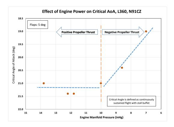
Figure 4, Effect of Propeller Thrust on Critical angle of Attack
