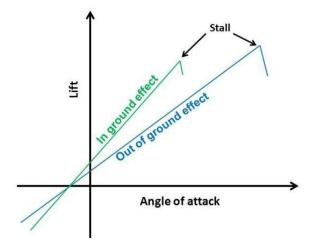
Figure 3, Critical AoA Change in Ground Effect, from NTSB report on G-650 accident
