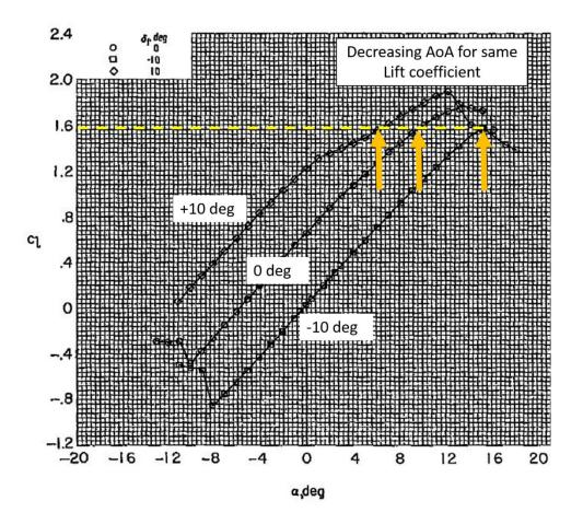
Figure 2, Effect of Flap Deflection on AoA at constant CL, NASA TP-1865
