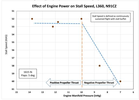
Figure 5, Effect of Propeller Thrust on Stall Speed
