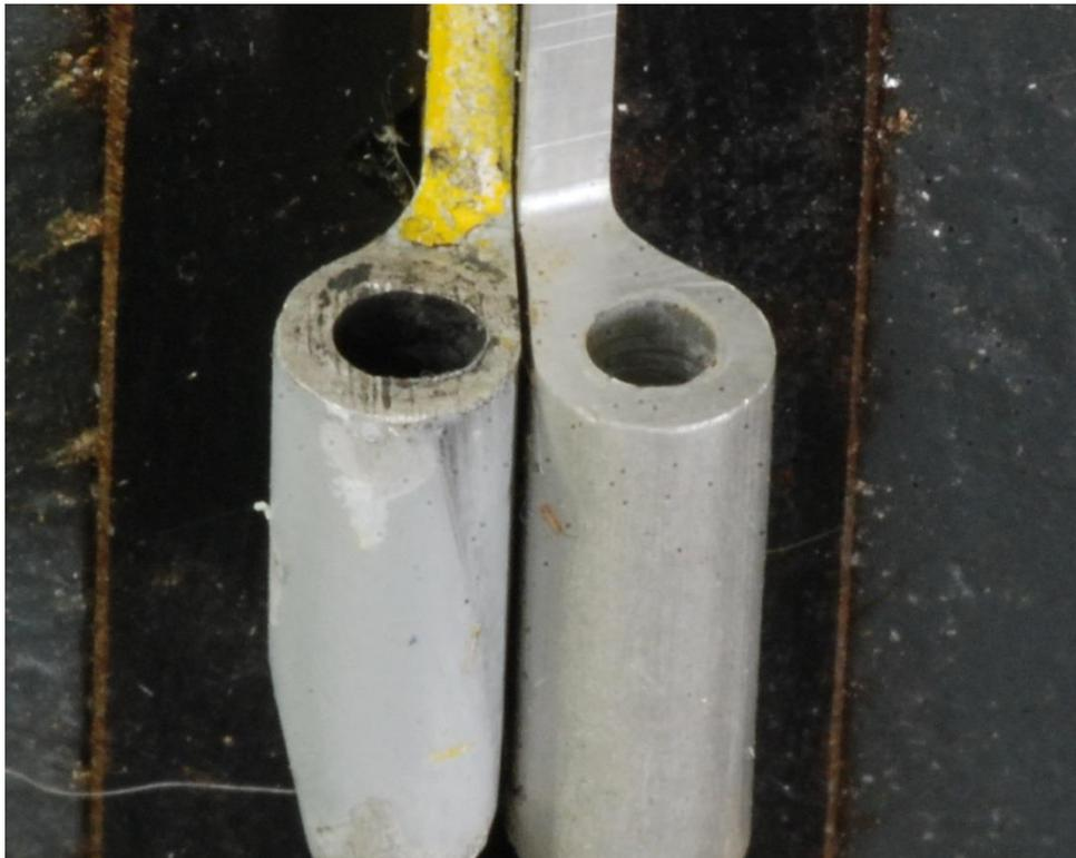
**Figure 1, Worn vs. New Hinge Material**
