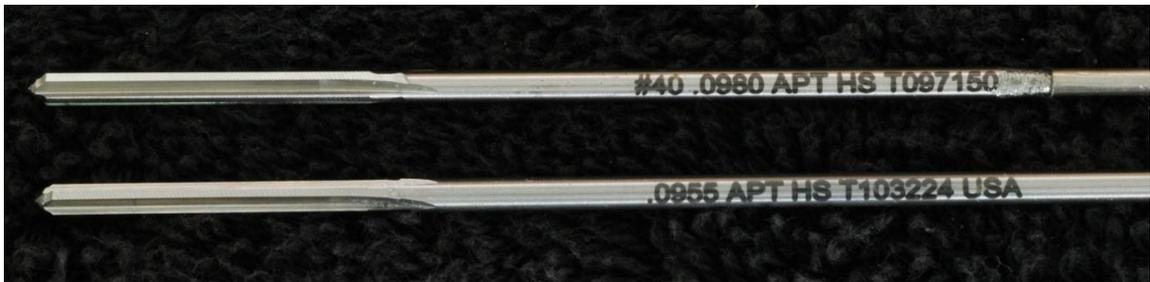
Figure 10, Reamers for making close tolerance MS hinges
