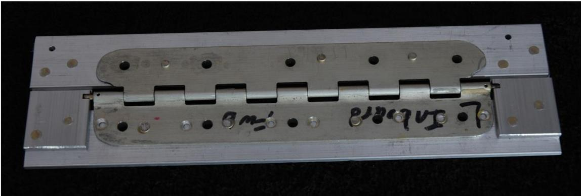
Figure 7, Completed hinge jig
