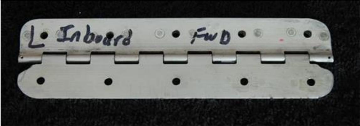
**Figure 2,** Used and worn MS hinge as removed from the aircraft
