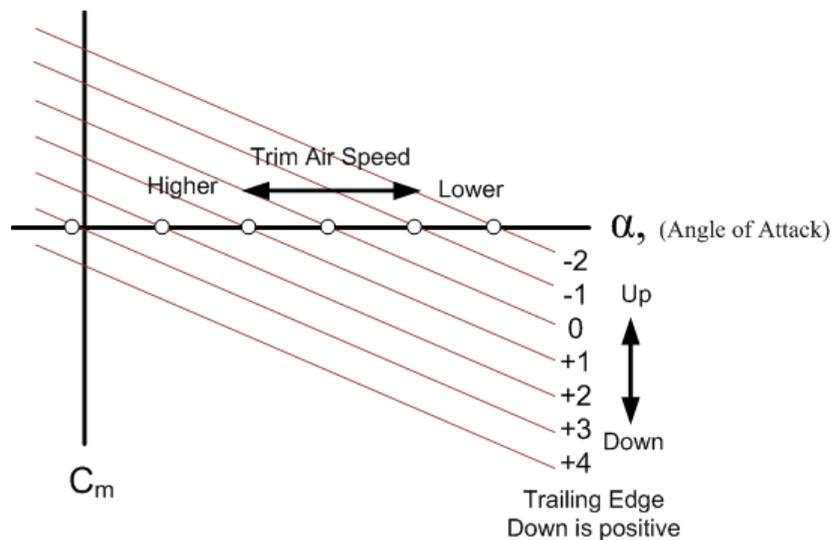
Figure 5, Effect of Elevator Deflection on Trim Speed
