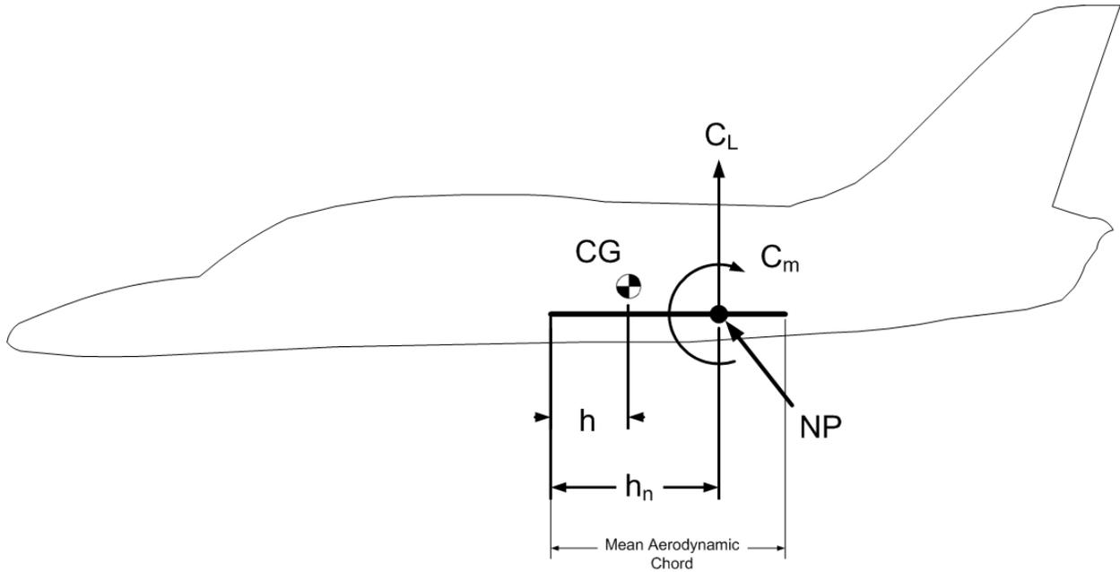
Figure 2, Total Lift and Moment acting on aircraft
