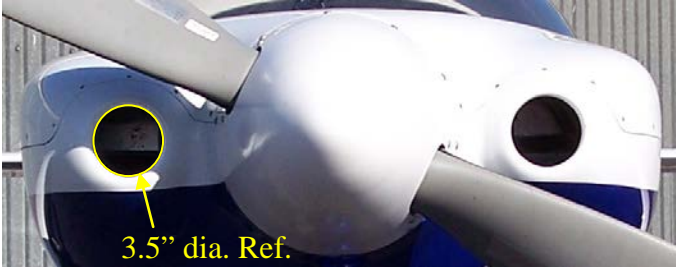
New Cowling – Inlets isolated from cowl split line
