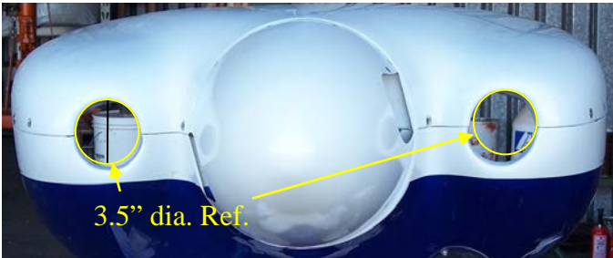
Original Cowling – Inlets ob-long to keep spinner opening round
